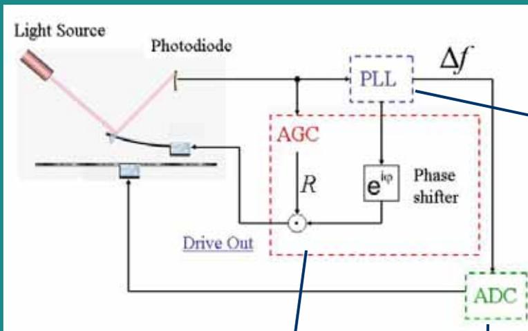
A complete, real time simulation of the entire NC-AFM experiment, including noise.
