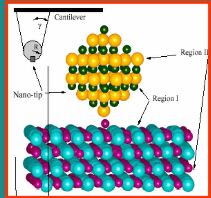
It is assumed that the instrumentation works ideally, the tip trajectory is periodic and that the tip-surface interaction is **conservative**
