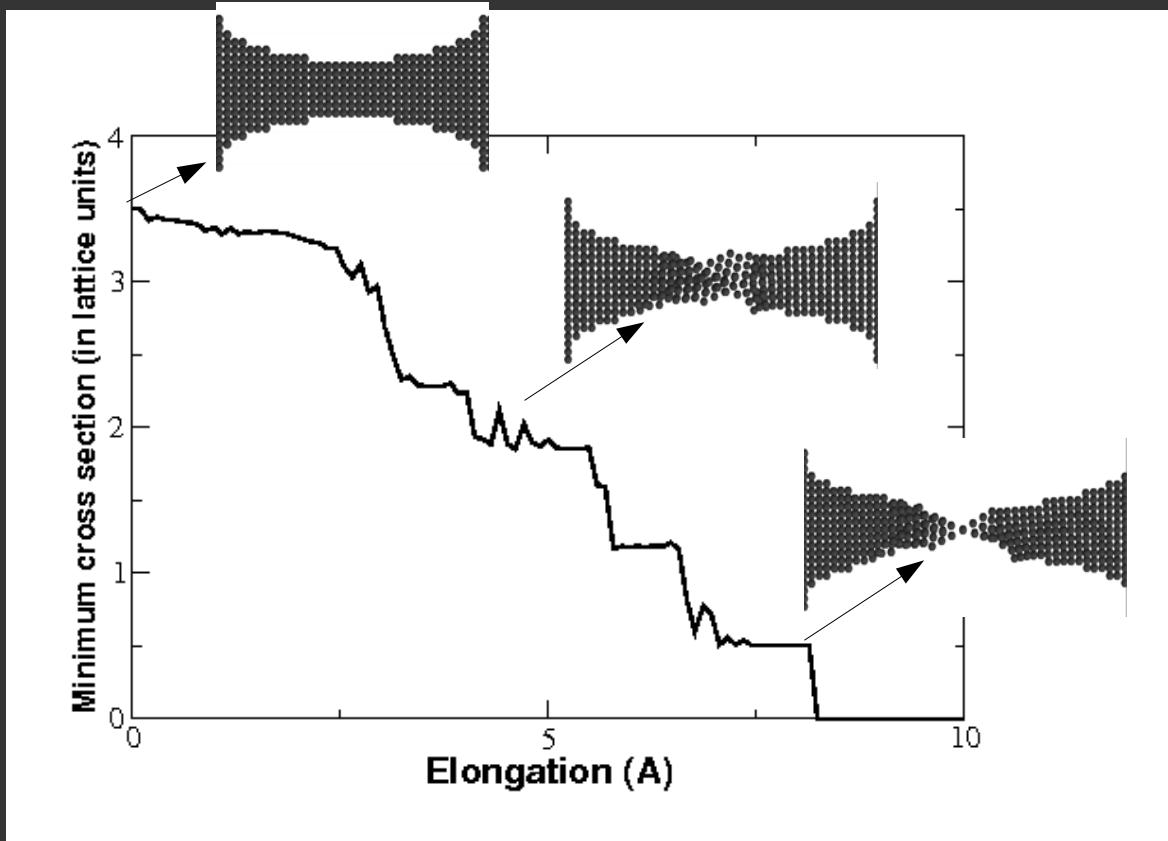
The smallest cross section is computed during elongation for 25 different cases
