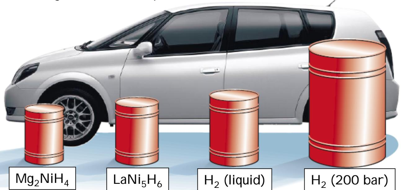
Volume of 4 kilograms of H (energy-equivalent to ~ 12 (or 24) kg of gasoline)
