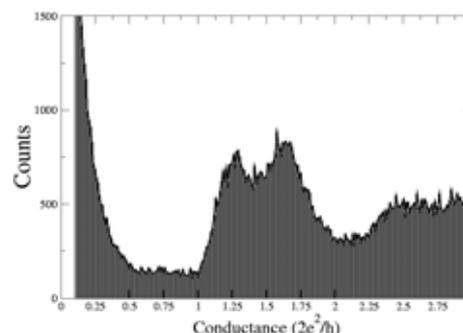
Figure 1: Experimental conductance histogram for Ni nanocontacts recorded at a bias voltage of 100 mV and a temperature of 4.2 K where two low conductance peaks are clearly visible.
