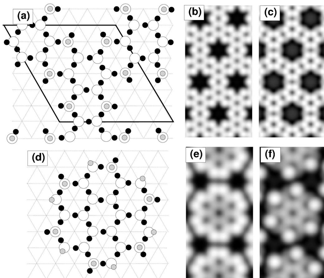
Figure 2: Optimized 2D water structures on Pd(111) for (a) lace and (d) rosette patterns. (b), (e) STM topographic image simulations for each model. (c),(f) Same as (b) and (e), but for models where the bridging species are OH species.
