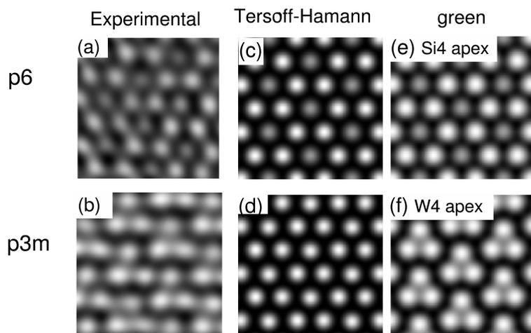
Figure 1. STM images for the  $Y_3Si_5(0001)$  surface. (a), (b) Experimental topographic images exhibiting p6 and p3m symmetry;  $I=1$  nAmp,  $V=-50$  mV. (c),(d) Tersoff-Hamann images evaluated 3 Å above the surface for the p6 and p3m models. (e),(f) Theoretical topographic images calculated with a tip (GREEN code)
