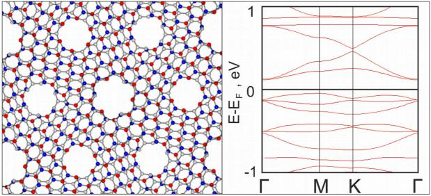
Fig. Semicoductor h-BN-graphene nanomesh and its band structure. Eg=0.18 eV
