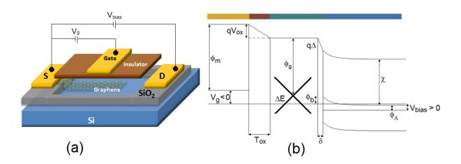
Figure 1.(a) Scheme of the Graphene Barristor proposed by Samsung in Ref. [2]; (b) Band diagram along a vertical cut along the gate stack.
