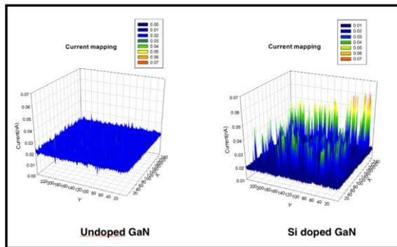
Figure2: Compare different doping concentration piezoelectric output current shown in the 3D graph.
