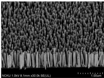
Figure1: Vertically aligned GaN NW array grown on the Si substrate. Side-view SEM images.
