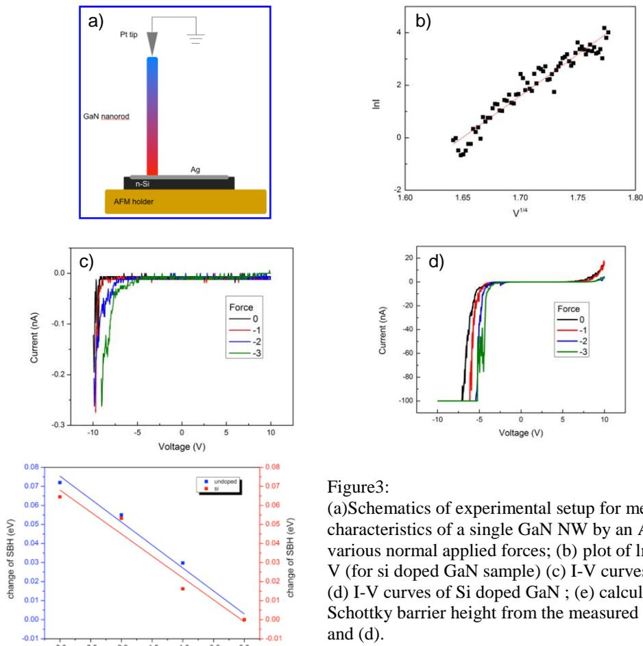
Figure3: (a)Schematics of experimental setup for measuring I-V characteristics of a single GaN NW by an AFM tip under various normal applied forces; (b) plot of  $\ln |I|$  as a function of  $V$  (for si doped GaN sample) (c) I-V curves of undoped GaN; (d) I-V curves of Si doped GaN ; (e) calculated change in Schottky barrier height from the measured I-V curves in (c) and (d).
