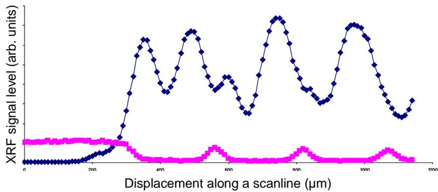
Figure 1 : Fe (blue) and Mo (pink) signals recorded along a scan line on the sample.
