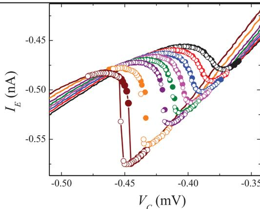
Figure 2: The effect of  $I_B$  on the  $I$ - $V$  characteristics of BOT. With increasing  $I_B$ , it clearly shows the approach towards bifurcation (right to left).
