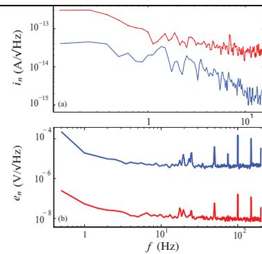
Figure 6: Input referred current noise ( $i_n$ ) in the current gain mode: red trace displays in with  $\beta_E = 1$ . The blue curve depicts  $i_n$  measured at  $\beta_E = 35$ . b) Input referred voltage noise ( $e_n$ ) in the transconductance mode: the blue curve is obtained at  $g_m = 10$  nS while the red trace was measured at  $g_m = 10$   $\mu$ S.
