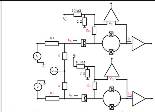
Figure 4: Measurement scheme used for measured of CMRR.
