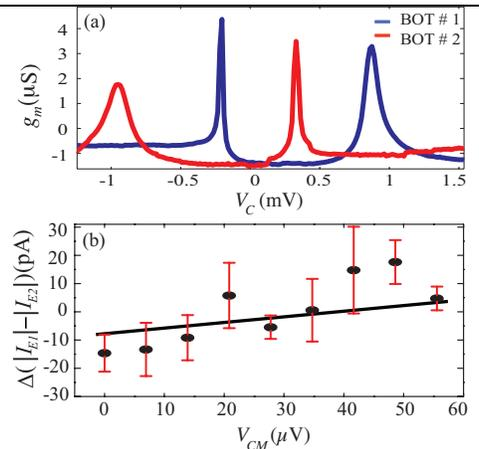
Figure 5: (a)  $g_m$  of the BOTs vs. collector bias  $V_C$ . (b) Difference of absolute output currents of the BOTs plotted vs. voltage applied to the CM port. Straight line yields a CMRR of 20dB.
