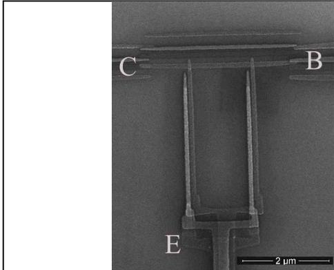
Figure 1: Scanning electron micrograph of a BOT. Collector, base and emitter are designated by C, B and E.
