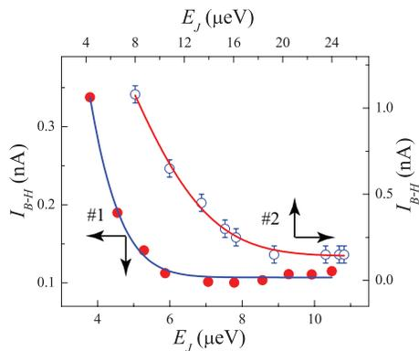
Figure 3: Bifurcation threshold over the  $I_{B-H} - E_J$  plane. #1 and #2 correspond to two samples measured in our experiment. Arrows denote the axis.
