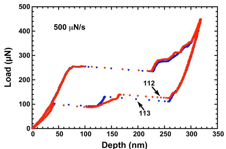
Figure 2: Nano-compression cycling in the Cu-Al-Ni micro pillar of Figure 1, performed in a Hysitron TI-950 instrumented nanoindenter. Reproducible behavior, showing two consecutive cycles numbered as 112 & 113.
