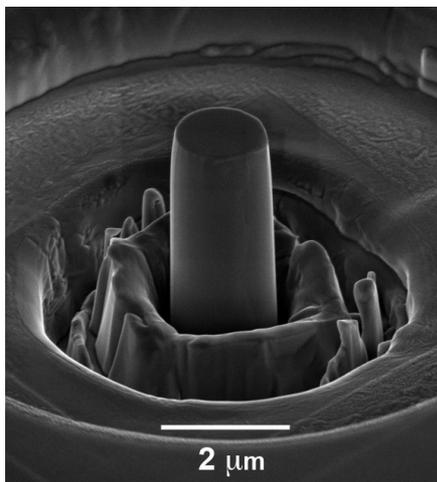
Figure 1: Micropillar of Cu-Al-Ni SMA milled by FIB on a [001] oriented single crystal, for nano-compression tests.
