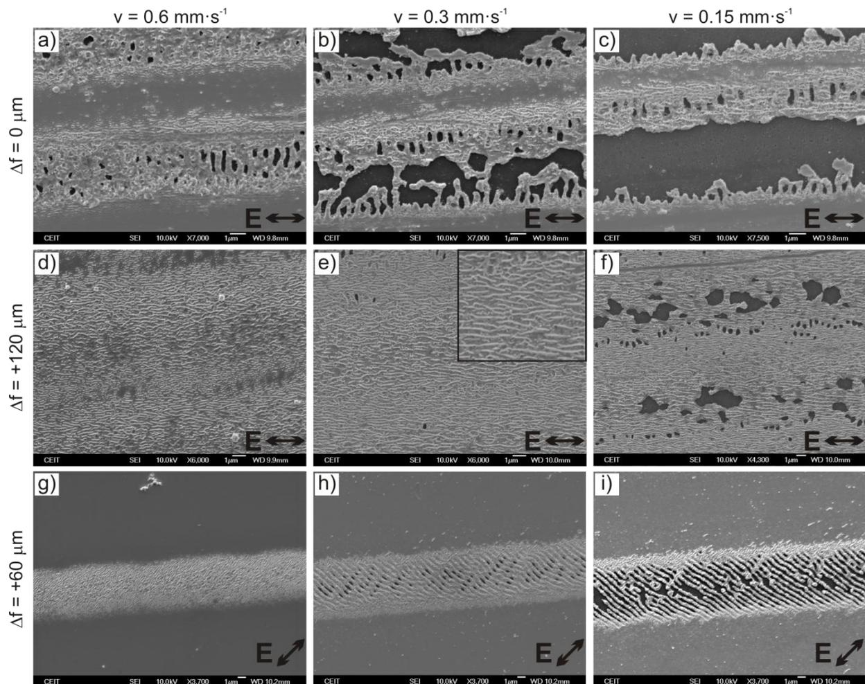
**Figure 1.** FE-SEM micrographs of the resulting LIPSS on Pt films for different irradiation conditions and horizontal displacement of 10 μm.
