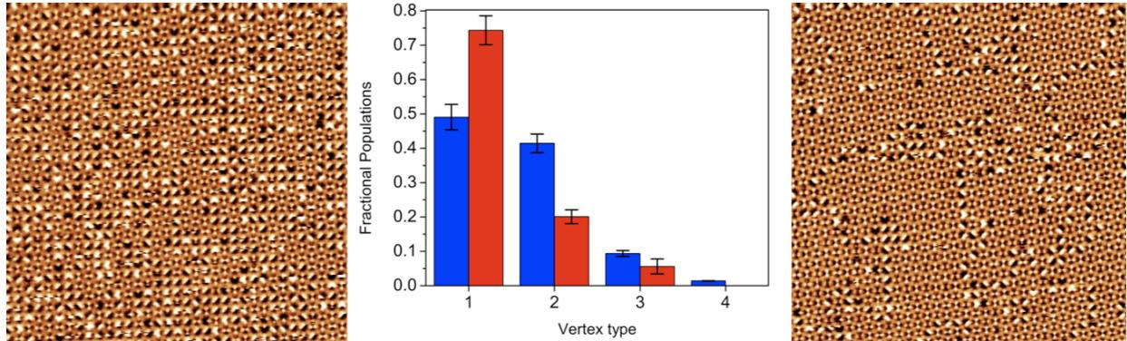
Fig.1: magnetization states after applying a sample-rotating in-plane magnetic field demagnetization protocol (left) and after melting the artificial spin-ice pattern over its blocking temperature (right), and a graphic of the vertex type populations (1-less energetic, 4-most energetic) obtained with the field demagnetization protocol (blue) and the thermal demagnetization protocol (red).
