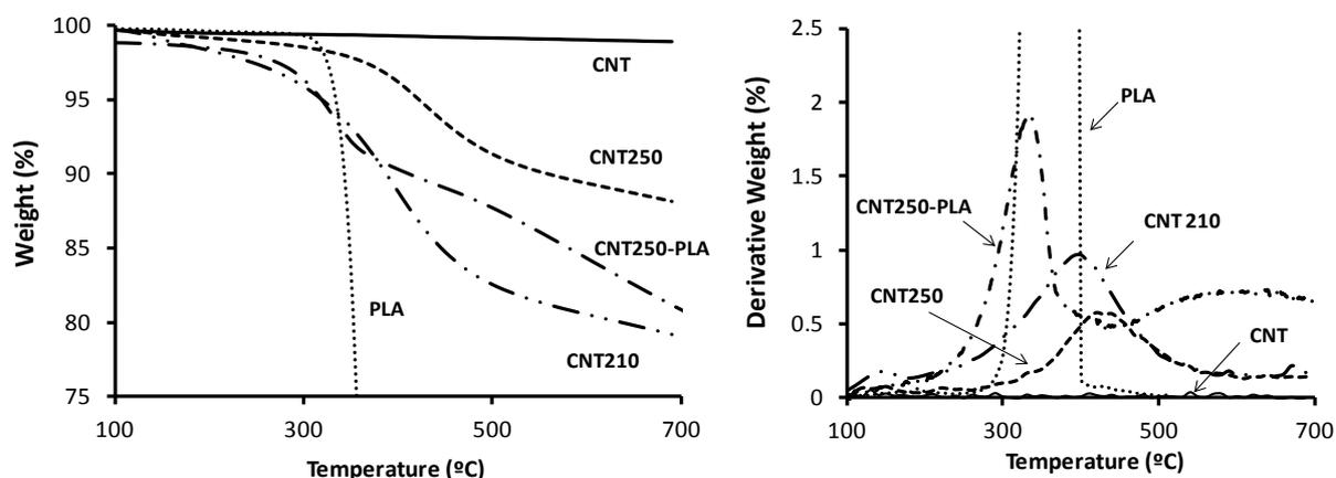
Figure 1. TGA curves of as-received CNT, functionalized CNT and PLA.
