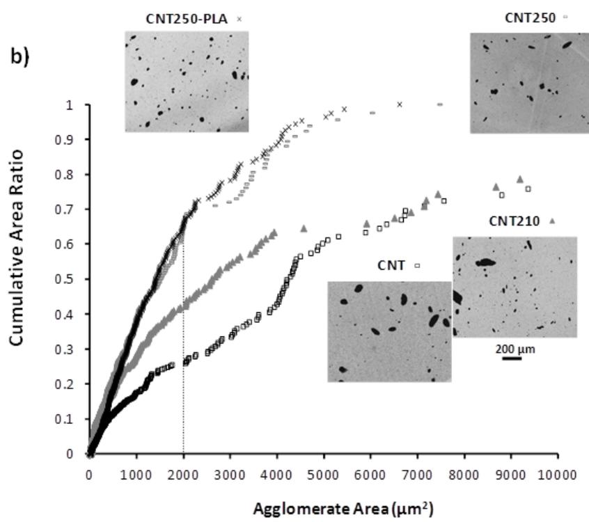
Figure 2. a) Electrical resistivity for PLA composites with non-functionalized and functionalized CNTs and b) cumulative area ratio for 2.0 wt% composites. The insert optical micrographs illustrate the observed agglomerate dispersion.
