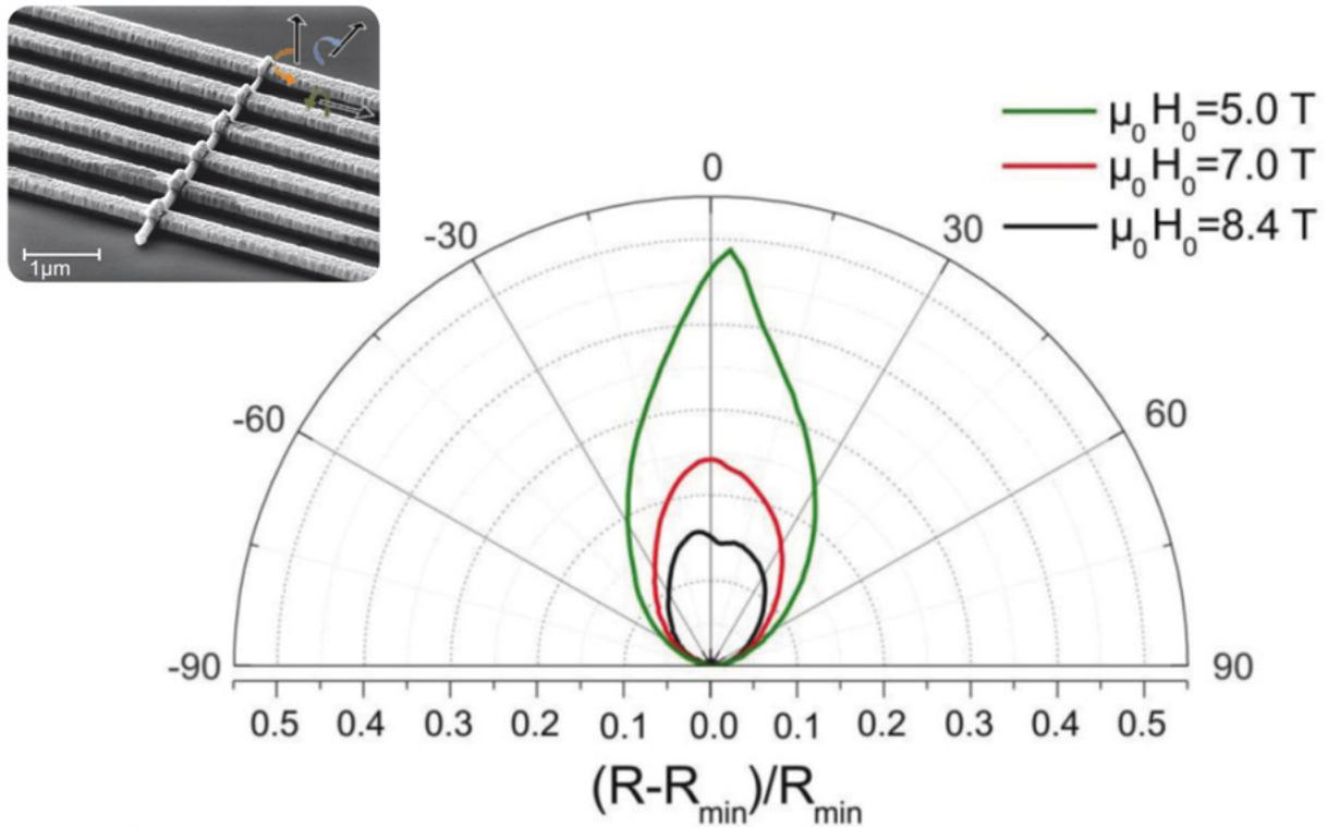
**Figure 1:** Normalized magnetoresistance as a function of the angle between externally applied magnetic field and the nanowire axis for various magnitudes of the external magnetic field. Inset (top left): Tilted scanning electron micrograph of a contacted nanowire. Black arrows indicate the sample coordinate system. Coloured arrows indicate the different rotational directions as used in the measurements (blue: transverse, orange: in-plane, green: perpendicular rotation).
