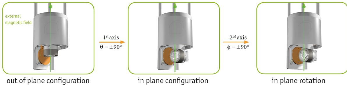
**Figure 2:** Working principle of the double rotator module and possible relative orientations between external magnetic field vector and sample surface.
