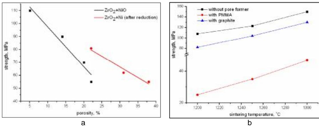
Figure 3. Strength of anode material vs porosity (a) and strength of cathode material vs sintering temperature (b)
