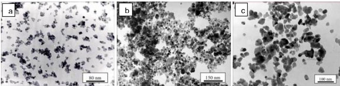
Figure 2. Structure of nanopowders  $\text{ZrO}_2\text{-8mol\%Y}_2\text{O}_3$ , NiO and LSMO for SOFC anode and cathode
