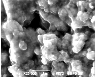
Figure 1. Structure of film based on  $\text{La}_{0.7}\text{Sr}_{0.3}\text{MnO}_3$  and  $\text{ZrO}_2\text{-3mol\%Y}_2\text{O}_3$  nanopowders
