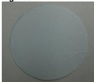
Figure 1. Photograph showing a circular PC sample without beads (47 mm in diameter) successfully extracted from the Al foil.
