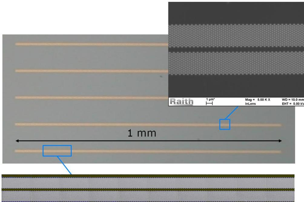
Figure 3. Hexagonal array of a 1mm-long, stitching error free photonic crystal waveguide written with MBMS stage technology.
