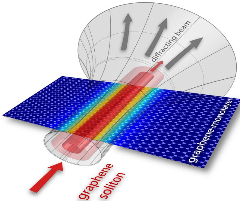
Schematic representation of the soliton formation by the intrinsic nonlinearity of the graphene monolayer (red cylinders). The gray surface displays the diffracting beam in the low power regime.
