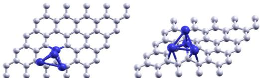
Fig. Top and side view of a tetrahedral Pd<sub>4</sub> cluster attached to a vacancy of graphene.
