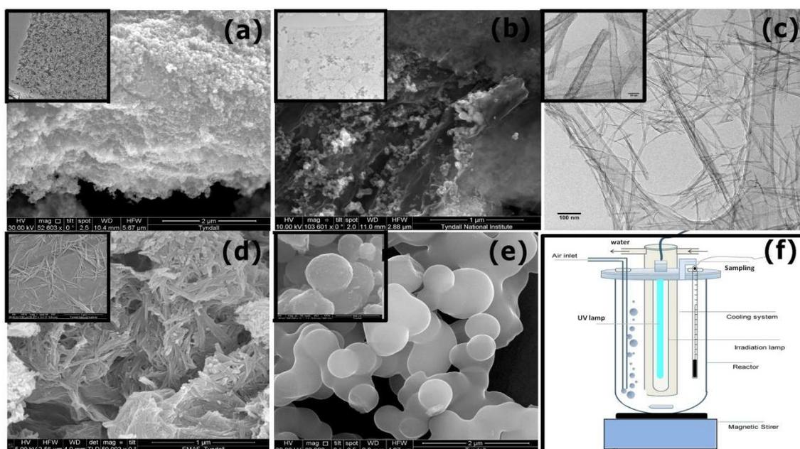
Figure 2: SEM and TEM images of (a) sol-gel synthesised TiO<sub>2</sub>/GO, (b) solution mixing of P25/GO, (c): in-situ hydrothermally synthesised TiO<sub>2</sub> nanotubes on RGO, (d): hydrothermally synthesised TiO<sub>2</sub> nanofibres/GO, (e): 3D network of TiO<sub>2</sub> beads/GO, (f): schematic image of immersion well Photocatalytic reactor
