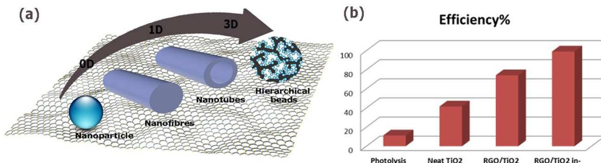
Figure 1: Dimensionality of TiO<sub>2</sub>/graphene composite (a), the effect of synthesis method on photocatalytic efficiency (b)
