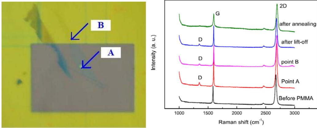
Figure 1. Left: Optical microscope image of graphene with e-beam lithography. Point A is the exposure part of graphene and point B is unexposure part. Right: Raman spectra for different conditions (1) before spin coating PMMA; (2) measurement of point A; (3) measurement of point B; (4) after lift-off with acetone; (5) after annealing
