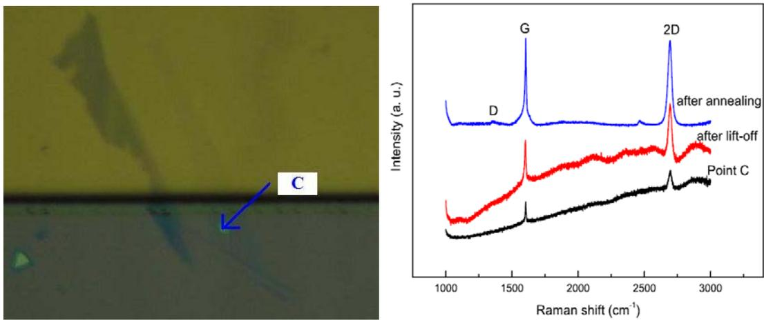
Figure 2. Left: Optical microscope image of graphene with photo lithography, Point C is the exposure part. Right: Raman spectra for different conditions (1) measurement of point C; (2) after lift-off with acetone; (3) after annealing.
