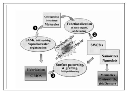
**Molecules in nanoelectronics:** Nano-objects can be categorized in 3 classes, molecules, carbon nanotubes, nanowires & nanodots. Molecules can be directly integrated in C-MOS devices (route 1) or for the functionalization of NObs (route 2) or/and for the preparation of receiving surface allowing the positioning of naked or functionalized NObs (route 3).
