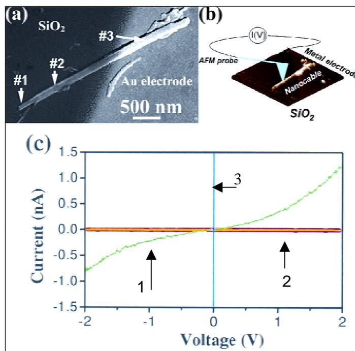
**Figure 2.** (a) SEM image of a semiconducting SiC nanowire protruding from an insulating BN nanotube; (b) AFM measurement set-up; (c) *I-V* curves taken at various spots: 1-SiC wire; 2-BN shielding tube; 3- Au electrode.
