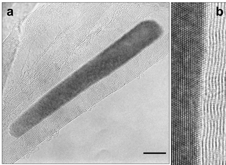
**Figure 1.** (a) HRTEM image of a C nanotube filled with a ferromagnetic FeCo alloy nanowire; and (b) enlarged view of the tube-filling interface displaying clear atomic steps on the filling. Scale bar in (a) is 5 nm.
