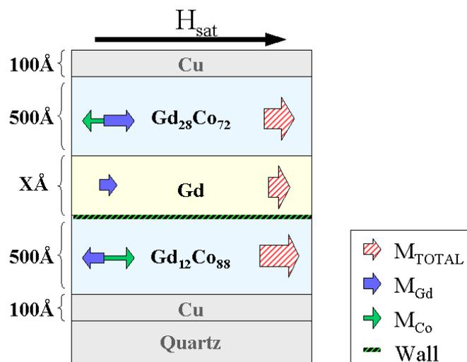
**Fig. 1.** Sample sketch where total magnetic moment of each monolayer is represented, as well as the magnetic moment of Gd and Co sublattices.
