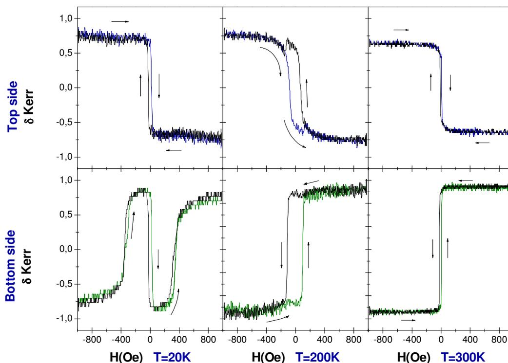
**Fig. 2.** T-MOKE hysteresis loops along the easy axis of both sides of  $\text{Gd}_{28}\text{Co}_{72}/\text{Gd}/\text{Gd}_{12}\text{Co}_{88}$  with  $35\text{\AA}$  Gd interlayer. Note that T-MOKE signal is only sensitive to Co moments. Arrows indicate the sense of the loop.
