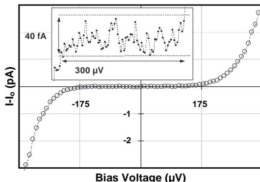
**Fig. 2** : Current step measured ( $f=10 \text{ MHz}$ ) obtained with R-pump provided by PTB (European project COUNT). Y-axis represents current deviation from zero bias voltage current. IV curve is fitted by an exponential function taking into account pumping errors. In insert, the plateau of measured current enlarged in the  $-200 \mu\text{V}/130 \mu\text{V}$  range.
