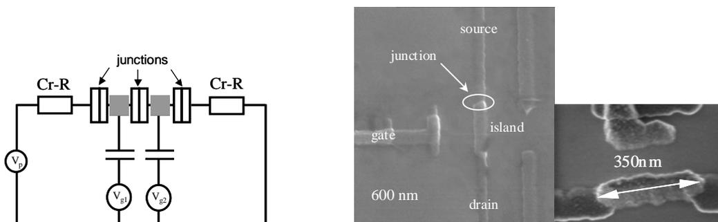
**Fig. 1** : On the left, a schematic view of a R-type 3 junctions pump, consisting of a chain of 3 tunnel junctions coupled through capacitors to gate voltages. On the right, a SEM image of a SET device with 2 junctions, with a enlarged picture of an island.
