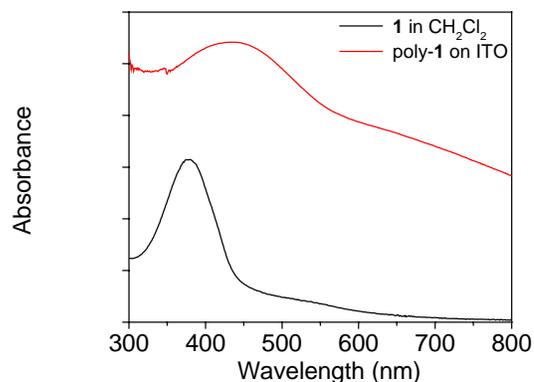
**Figure 3.** UV-Vis absorption spectra of **1** and poly-1.
