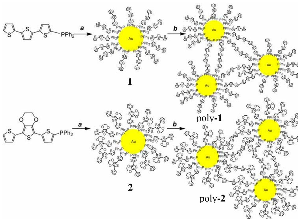
**Figure 1.** Preparation of oligothiophene-linked Au nanoparticles.  $\text{HAuCl}_4$ , Toluene,  $\text{H}_2\text{O}$ ,  $[\text{N}(\text{C}_8\text{H}_{17})_4]\text{Br}$  followed by addition of 15 equiv of  $\text{NaBH}_4$  at room temperature. <sup>b</sup>Electrodeposition in  $\text{CH}_2\text{Cl}_2$  containing 0.1 M  $(n\text{-Bu})_4\text{NPF}_6$  on a Pt, ITO or Au working electrode.
