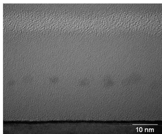
Figure 2. Cross-sectional bright field TEM image of sample C.
