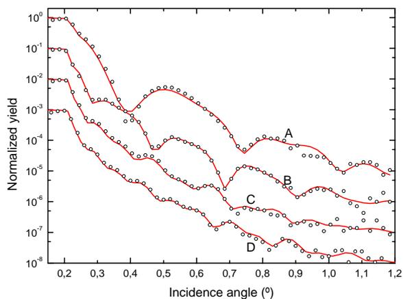
Figure 3. XRR spectra and their fit for the 4 samples.
