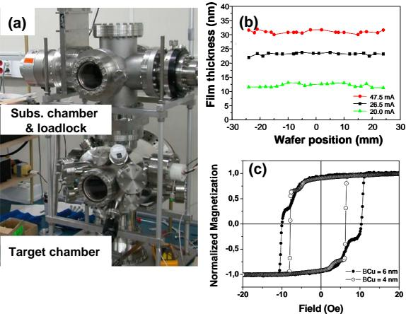
**Fig. 1**. (a) Image of the Ion-beam sputter system with labels for the upper and lower chambers. (b) Thickness variations over a 5cm-diameter silicon wafer for NiFe films grown at beam-currents of 47.5 mA (full circles), 26.5 mA (full squares) and 20 mA (full triangles), respectively. (c) Room temperature MOKE hysteresis loops showing distinct layer switching for NiFe (6 nm)/ Cu (6 or 4 nm)/ CoFe (6 nm) pseudo-spin-valves.
