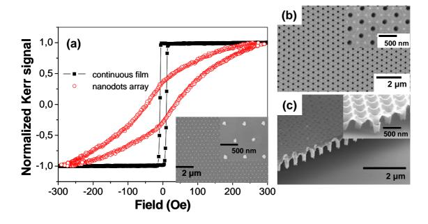
**Fig. 2**. (a) Moke hysteresis loop probing a 2.8 μm-diameter area of a NiFe array of nanomagnets with lateral dimension of 120 nm and thickness of 13 nm. The inset show scanning electron micrographs (SEMs) of the array with different magnifications. (b) Plan-view and (c) side-view SEMs corresponding to membranes used as shadow-masks.
