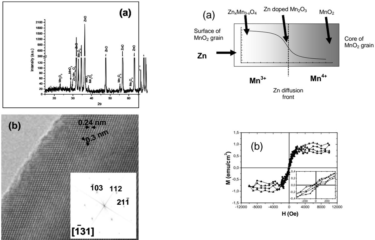
**FIG. 2:** (a) Scheme of the different phases at the Mn oxide grains after annealing at 500°C and the oxidising states of Mn. The graph indicates the concentration profile of Zn inside the grain. (b) Hysteresis loops from a 40 MnO<sub>2</sub>/ZnO multilayer prepared by laser ablation at 5K (triangles) and 300 K (circles). Inset shows a detail of the loops at low  $H$ . The paramagnetic/diamagnetic component has been subtracted to clearly show the FM phase.
