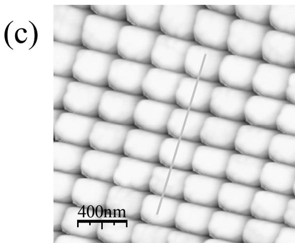
AFM image of photoresist mask with bits pattern prepared by SEM photolithography
