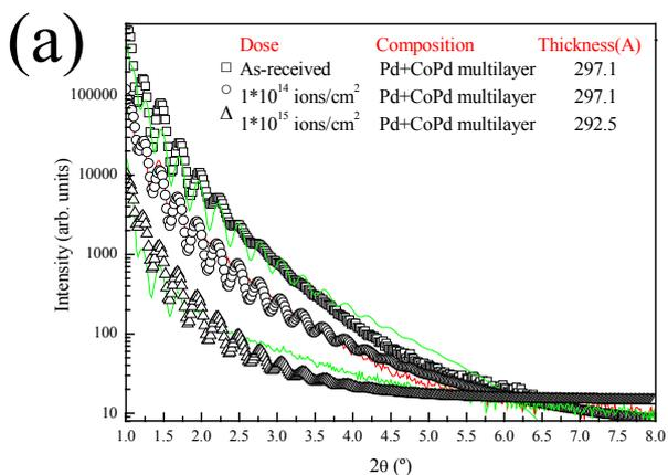
Glancing angle X-ray reflectometry of the sample as received and after implantation with different doses. No big change in the thickness is observed.
