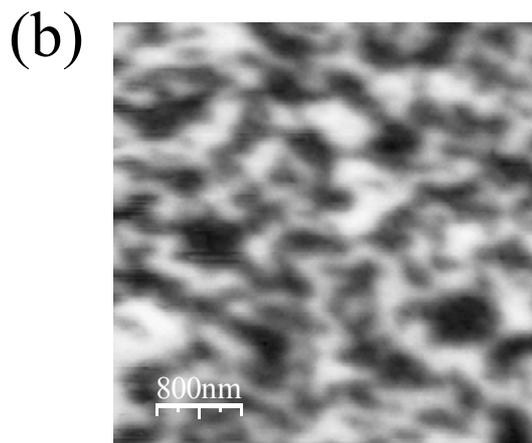
MFM Image of magnetic domains of the as-received sample in a demagnetized state
