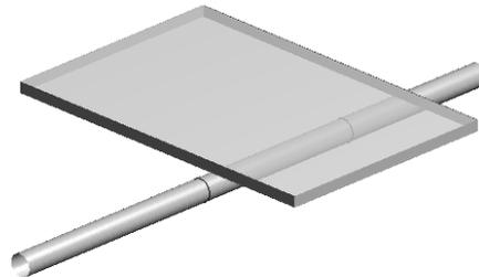
**Figure 1** - The model geometry considered in this work: a single carbon nanotube below a planar gate electrode. The portion of the nanotube directly below the gate is the undoped channel, and the doped source and drain are connected to it.
