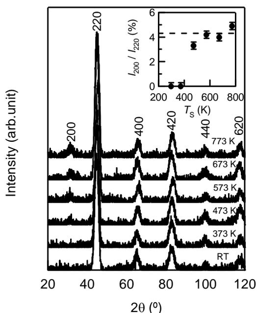
Fig. 1 X-ray diffraction patterns for  $\text{Co}_2\text{FeAl}$  (100-nm thick) films deposited on a thermally oxidized Si substrate with various temperatures. The inset shows substrate temperature dependence of the intensity ratios ( $I_{200}/I_{220}$ ). The dotted straight line indicates the calculated values assuming the perfect  $B2$  structure ordering in the films.
