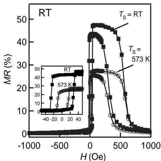
Fig. 2 Magnetoresistance curves at RT for MTJs with a  $\text{Co}_2\text{FeAl}$  film deposited at RT and 573 K. The corresponding crystal structures are the A2 and the B2 structures, respectively. The inset indicates the magnification of the magnetoresistance curves at low magnetic field region.
