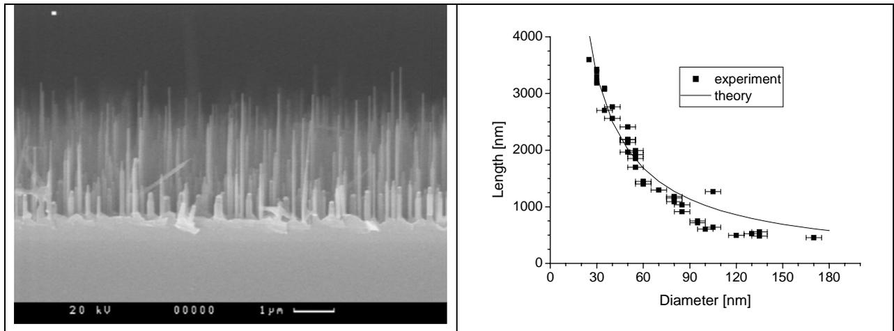
Fig. 1. SEM image, comparison of experimental and theoretical length/diameter dependencies for GaAs NWs
