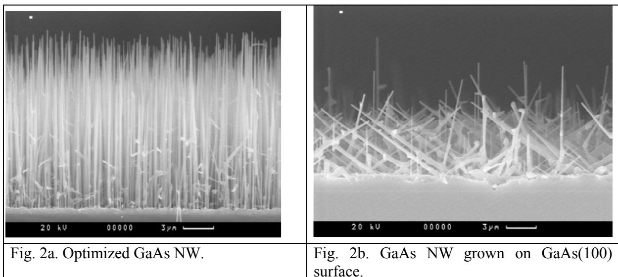
Fig. 2a. Optimized GaAs NW.
