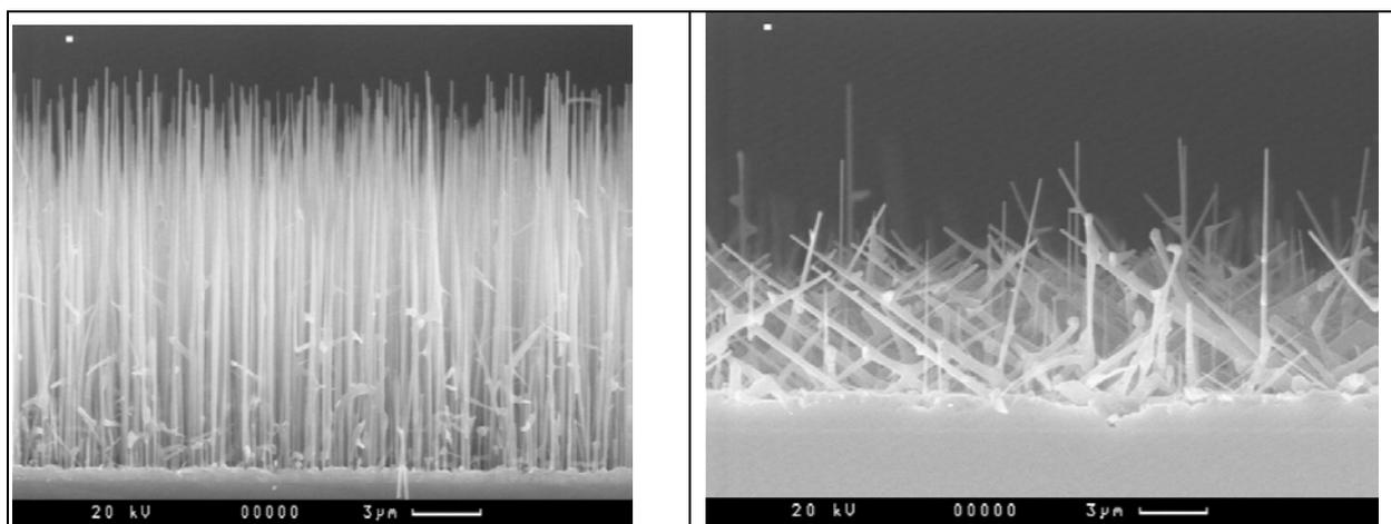
Fig. 2a. Optimized GaAs NW.
