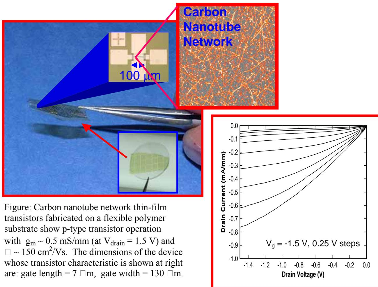
Figure: Carbon nanotube network thin-film transistors fabricated on a flexible polymer substrate show p-type transistor operation with  $g_m \sim 0.5$  mS/mm (at  $V_{\text{drain}} = 1.5$  V) and  $\square \sim 150$  cm<sup>2</sup>/Vs. The dimensions of the device whose transistor characteristic is shown at right are: gate length = 7  $\square$ m, gate width = 130  $\square$ m.
