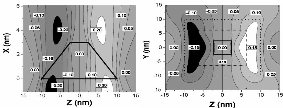
**Figure 1:** Contour plot of the total electrostatic potential (piezoelectric plus spontaneous contributions) for a truncated square-based-pyramid quantum dot in planes ZX ( $Y=0$ ) and YZ ( $X=1.5$  nm). The pyramid height is 3.0 nm. The labels over the contour show the magnitude of the potential in eV. The dark and bright areas correspond to the regions of low and high potential, respectively.
