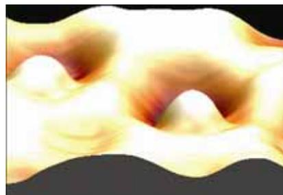
Fig 3: 3D AFM image of InAs QD nucleated in the GaAs nanoholes.
