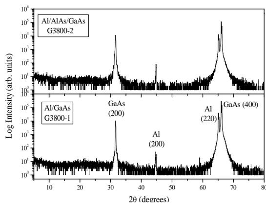
Fig 1: X-ray diffractograms of Al layer grown on AlAs/GaAs (top) and on GaAs (bottom) on silicon doped GaAs(001) substrates. The diffractograms show the coexistence of Al (110) and (100) crystallographic orientations.
