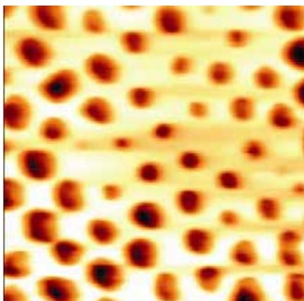
Fig 2: 1x1  $\mu\text{m}^2$  AFM image of patterned GaAs surface after alumina removal
