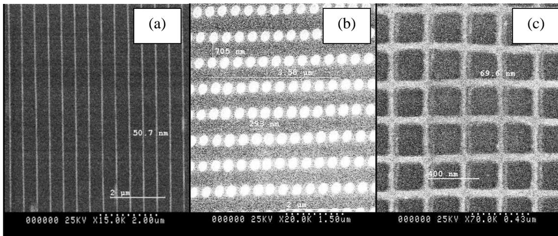
Fig.1. SEM images Si nanoprofiled substrates with different surface topography patterns: (a) lines, (b) dots and (c) lattice.
