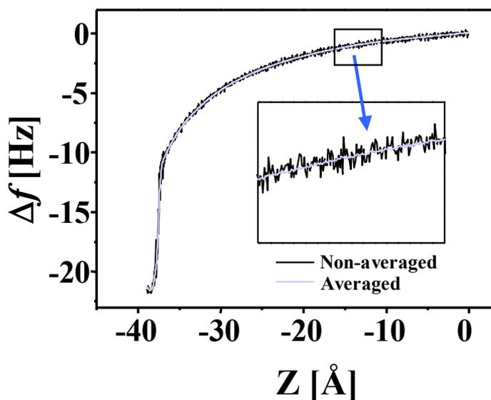
Fig.2 Averaged (grey solid line) and non-averaged (black solid line)  $\Delta f$ -z curves.
