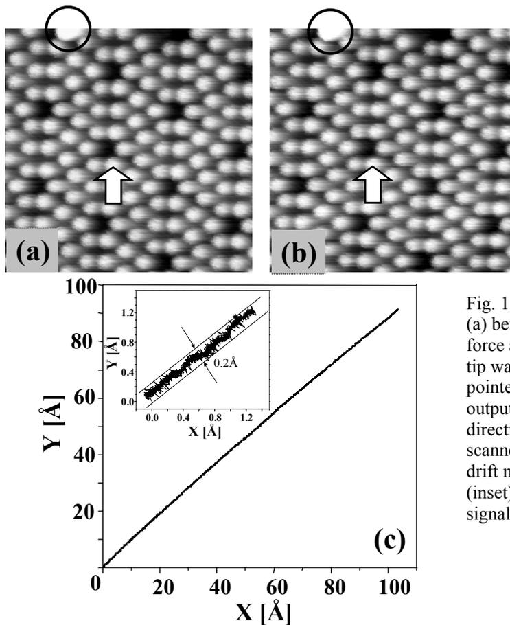
Fig. 1 NC-AFM topographic images of (a) before and (b) after 61 minutes of force atom tracking, respectively. AFM tip was fixed on the corner adatom pointed by the arrow. (c) Feedback output signals in the orthogonal directions (X and Y) of the piezoelectric scanner for compensating the thermal drift movement in the lateral direction. (inset) Zoom of the feedback output signals in X and Y directions.
