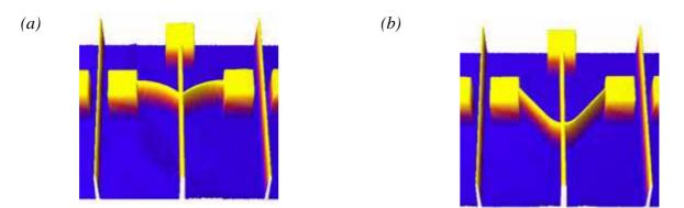
*Figures 2* Interferometric image of the hydrodynamic focuser masters used in the imprint process. In both cases the channel height is 5  $\mu$ m and the width 50  $\mu$ m.
