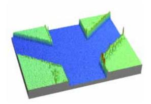
*Figure 3* Interferometric image of the central part of the PMMA replica of the structure in figure 2(a). The replica follows tightly the master features.
