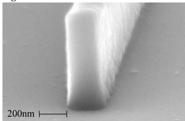
**Fig. 1:** SEM image (70° tilt view) of line pattern after development. Bottom line width 260nm, line spacing 1.81 $\mu$ m. Exposure area dose 220 $\mu$ C/cm<sup>2</sup>.
