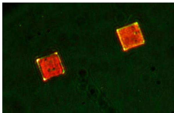
**Fig. 6:** Optical microscopy images of light transmitted through the coax arrays. Wavelength filtering effect observed at  $\lambda=650$ nm.
