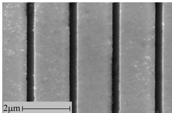
**Fig. 2:** SEM image (top view) of line pattern after lift off in ultrasonic acetone bath. Final line width 290nm, line spacing 1.81 $\mu$ m.
