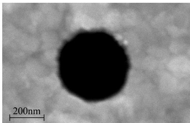
**Fig. 3:** SEM image (top view) of dots pattern after lift off. Final dot diameter 400nm, Exposure dose 250 $\mu$ C/cm<sup>2</sup>.
