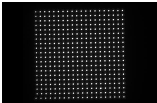
**Fig. 4:** Optical microscope image of white light transmission through a 20x20 array of holes of 400nm diameter.
