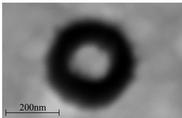
**Fig. 5:** SEM image (top view) of a coax after lift off. Exposure dose 250 $\mu$ C/cm<sup>2</sup>.
