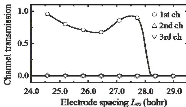
Fig. 2: Channel transmission at the Fermi level for the optimized three-aluminum-atom wire as a function of electrode spacing.
