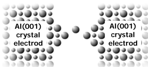
Fig. 1: Schematic representation of the aluminum nanowire model.
