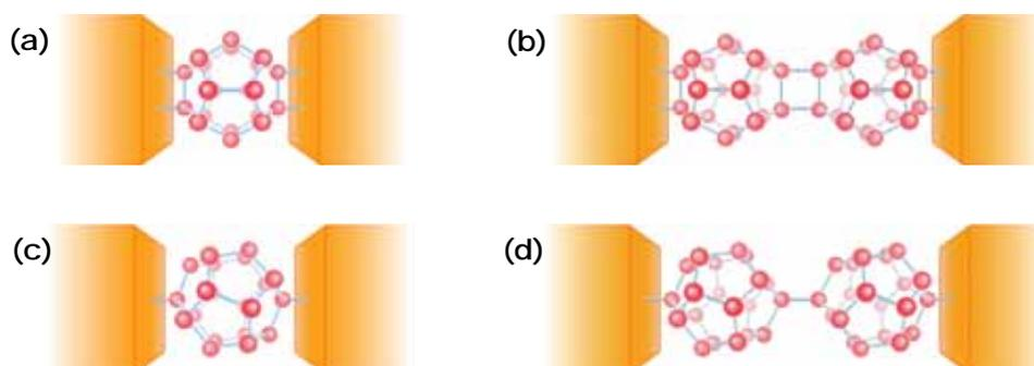
Fig. 4: Schematic descriptions of the scattering region of  $C_{20}$  suspended between Au electrodes: (a) double-bonded monomer, (b) single-bonded monomer, (c) double-bonded dimer, and (d) single-bonded dimer models.
