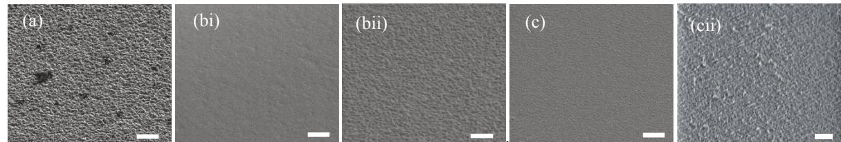
Fig. 2. SEM images of (a) the SnO<sub>2</sub> coated master, and the (i) pristine and (ii) hot embossed surfaces of (b) PMMA and (c) PEN (bar = 2  $\mu\text{m}$ ).
