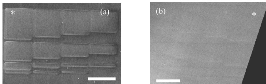
Fig. 3. SEM images of (a) the milled Si<sub>3</sub>N<sub>4</sub> master, and (b) PEN nanoimprinted surface (bar = 20  $\mu\text{m}$ ). The \* marks the position of the 20 x 20  $\mu\text{m}$  structure. (PMMA image unavailable at this time).
