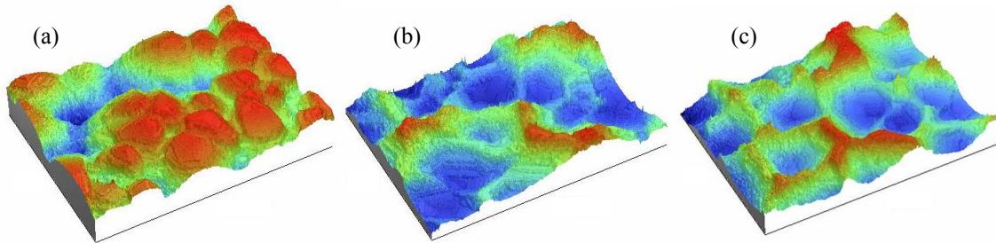
Fig. 1. White light interferometer images of (a) the frosted glass master, and (b) PMMA and (c) PEN hot embossed surfaces (image dimensions = 94.6 x 124.4  $\mu\text{m}$ ).
