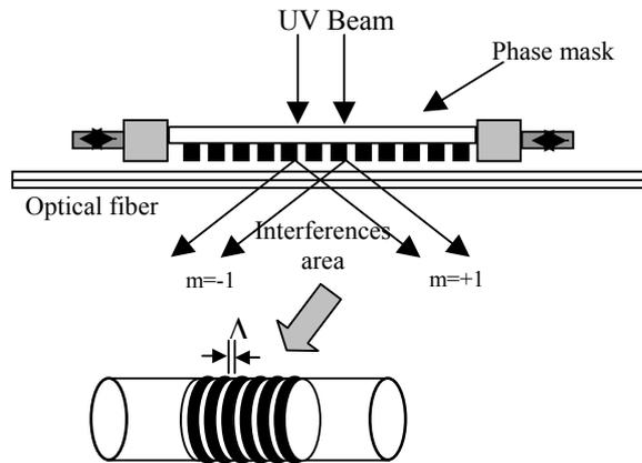
**Figure 1 : Typical assembly for the inscription of the index modulation in a photosensitive device**
