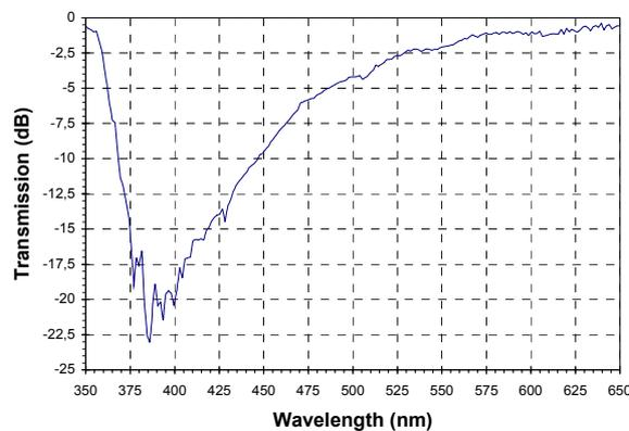
**Figure 3 : Slanted grating around 380 nm showing cladding and radiative modes in a SMF-28 fiber**
