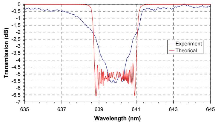
**Figure 2 : Correlation between the simulation and the experimental results for a 640 nm chirp grating**
