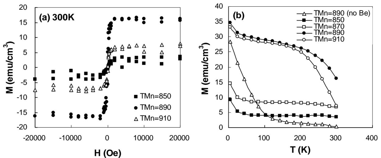
Fig. 1. M-H and M-T curves of the grown Be-codoped GaMnAs layers.
