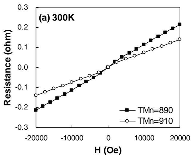
Fig. 2. Anomalous Hall effect measurements of the Be-codoped GaMnAs layers.
