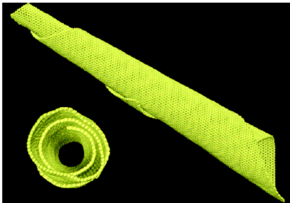
Figure 1. Three dimensional view of a Carbon Nanoscroll obtained from molecular dynamics simulations.
