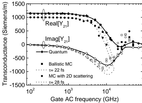
Fig 3: Transconductance frequency response. Symbols  $\circ/\square$ , MC with/without scattering. Solid line and  $\diamond$ , Quantum TDSE. Dotted lines correspond to the expected analytical response for different  $\tau$ .
