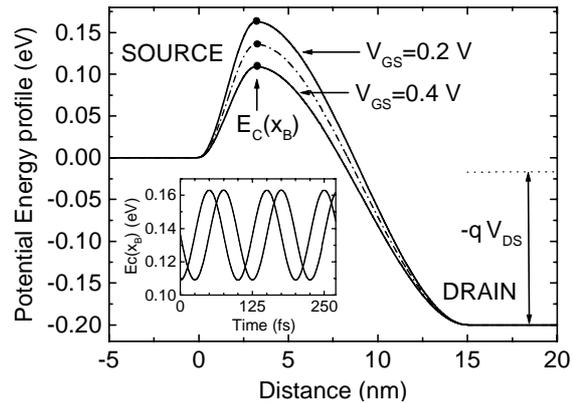
Fig 4: Oscillating (non-self consistent) energy potential profile Inset: Maximum of  $E_C(x,t)$  for a cos/sinusoidal oscillating gate voltage.
