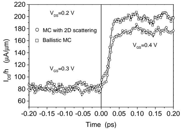
Fig 2: The MC (non-self consistent) results of the current transient response to a gate step voltage, 0.1V, while the  $V_{DS}$  is fixed.
