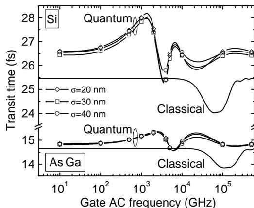
Fig 6: Classical and QM transit time as a function of the gate frequency. The shapes are different, but both values are quite similar and independent of the wave-packet dispersion  $\sigma$ , for a fixed (Si or AsGa) effective mass.
