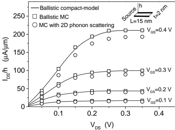
Fig 1: Current vs. voltage characteristics for the DG MOSFET. The MC results include energy quantization and 2D-degenerate injection.
