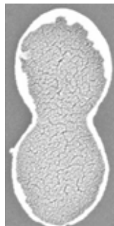
Fig. 1: SEM image of typical patterned particle, approximately 730 nm long with largest and smallest widths 320 nm and 200 nm, respectively.
