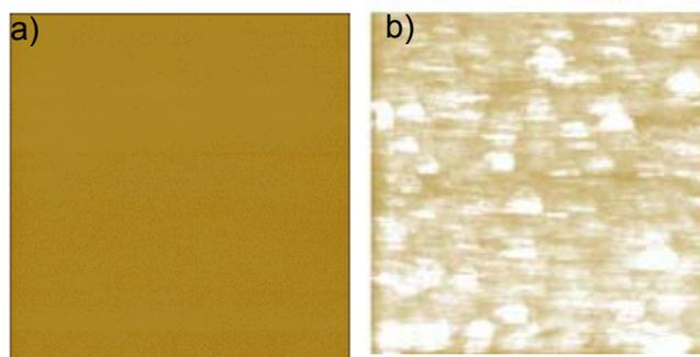
Fig. 1. Current maps of the gate stacks measured when applying a sample bias of 6V (substrate injection), a) not annealed sample, b)  $T_A=900\text{C}$ . The area of the scanned region is  $2\times 2\mu\text{m}^2$ . The current ranges from 0pA (black) to 20pA (white).
