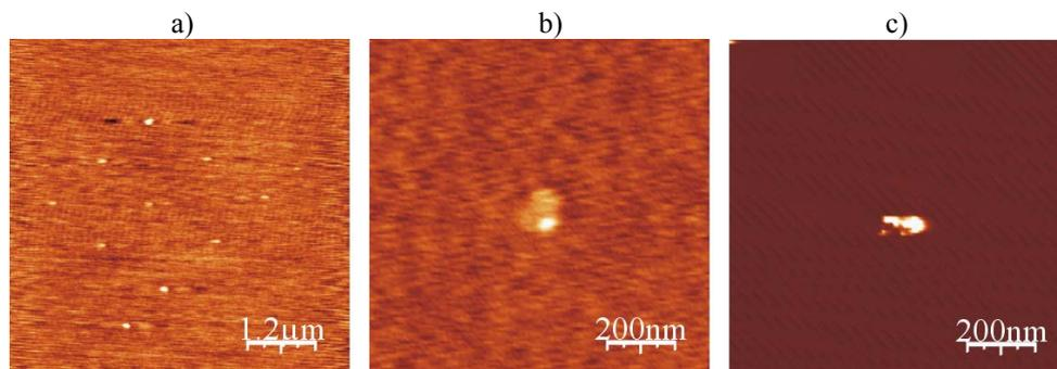
Figure 2. a) Topography map showing 10 hillocks measured at the location where RVS (0V up to 15V) were previously applied. Hillock height ranges from 1 to 6 nm. b) Topography and c) current maps ( $V_{\text{gate}}=3\text{V}$ ) corresponding to a zoom of one of the hillocks observed in a). Height range is from 0 (black) up to 6nm (white). Current range is from 100fA (noise level) (black) up to 300pA (white).
