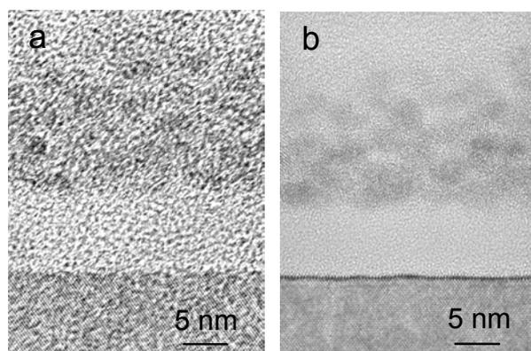
Figure 3. Cross-sectional bright field images of SiGe nanoparticles embedded in SiO<sub>2</sub>. a) Sample directly deposited by LPCVD on top of a 20 nm SiO<sub>2</sub> buffer layer. b) The same sample after SiGe crystallization.
