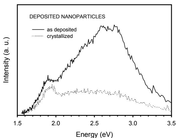
Figure 4 CL spectra of the SiGe/SiO<sub>2</sub> structures shown in figure 3. a) As-deposited. b) Crystallized.
